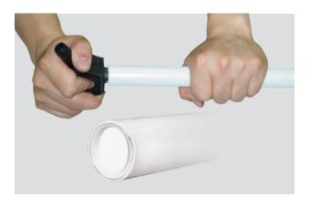
Step2: Round and bevel the ends with the RIIFO reamer
