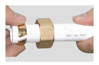
Choose the right size of the fitting according to the pipe; place the nut and then the compression ring onto the Please note the threaded opening must face the end of the pipe.
